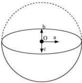
Since gravitational intensity at a point is defined as the gravitational force per unit mass at that point, it will also act in the downward direction. Thus, the gravitational intensity at centre O of the given hemispherical shell has the direction as indicated by arrow  $\mathbf{c}$ .
